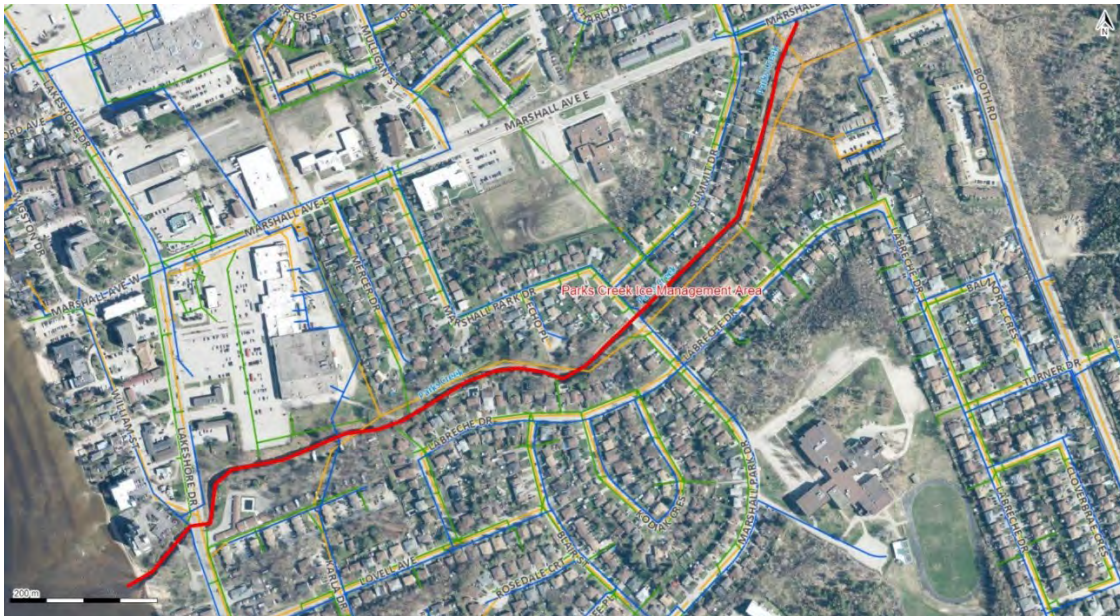
Figure 1 - Parks Creek Ice Management Area overview (red line) downstream of Marshall Ave to outlet with Lake Nipissing with municipal linear infrastructure. Blue line signifies watermain; green line signifies storm sewer; orange line signifies sanitary sewer.
